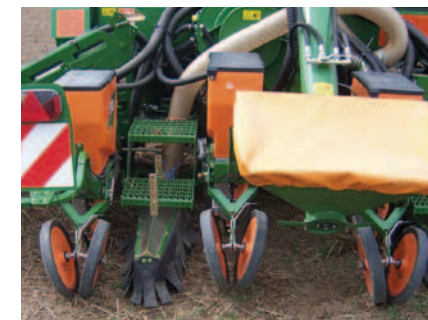
Sowing machine with exhaust air deflector
