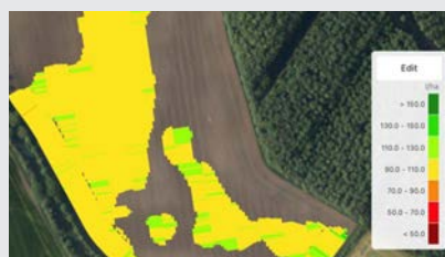
A spray application map can be created to target the patches of infested weeds only
