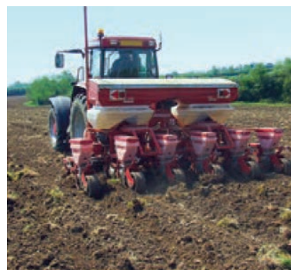
Drilling into trashy seedbed risks leaving seed on surface
