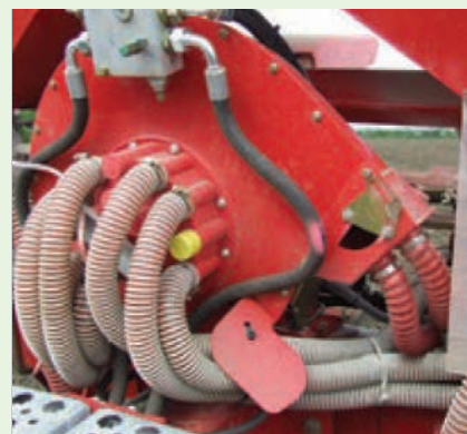
Vacuum drills must be manufactured or adapted to prevent dust being released into the air
